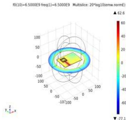
Fig. 3 : Electric Field (emw)
