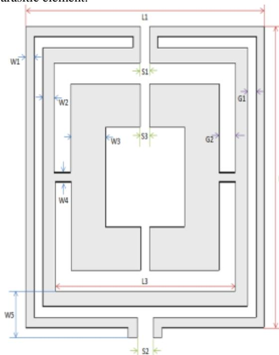
Fig.1 Antenna geometry
